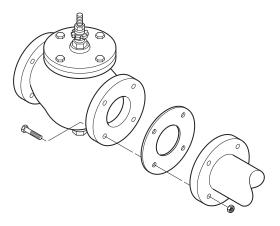
Figure-5 Installation of Flanged End Valves.
