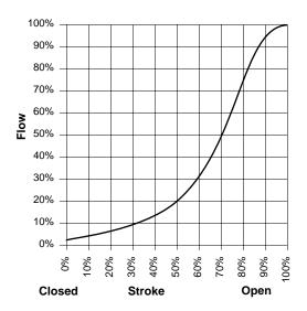
Figure-1 Typical Equal Percentage Flow Characteristics.
