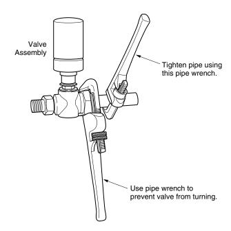
Figure-4 Installation of Screwed End Valves.
