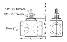
Figure-6 Typical of VB-9213-0-4-P, 2-1/2" and 3" Valve Bodies.
