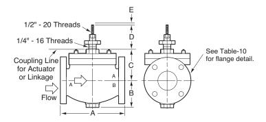
Figure-7 Typical of VB-9213-0-5-P 2-1/2" to 6" Valve Bodies.
